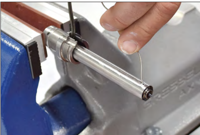
Picture 85: Installation of the new thermocouple
