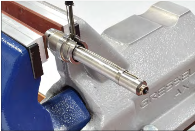
Picture 80: Clamp the nozzle
