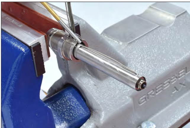
Picture 81: Pull off the clamping sleeves
