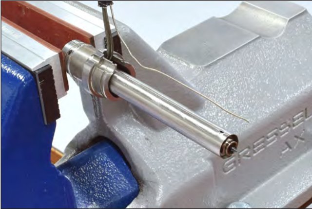
Picture 83: Disassemble the broken thermocouple
