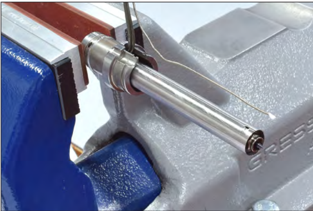
Picture 84: Coated tip of the thermocouple
