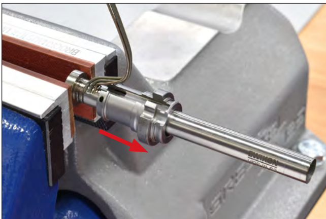
Picture 73: Pull off the nozzle body
