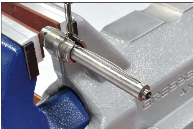
Picture 82: Pull out the protective tube
